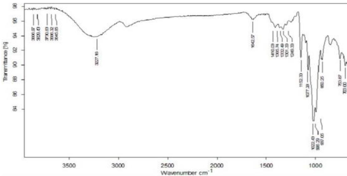
**Figure 4.2** FTIR spectrum of  $\beta$ -CD
