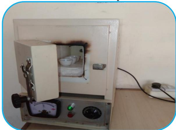
**Figure 5.** Muffle furnace
